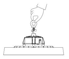
• Install the coarse wire or cable to the ceiling by screwing it or using a suspension kit for ceiling fixture installations.
