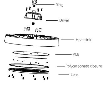
• Luminaire contains last technology protection screens for greater heat dissipation and greater work performance.
