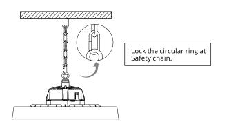
•Check that the fixing is correct before connecting the wiring. If the luminaire is held securely, proceed with the connection of the luminaire to the power supply.
